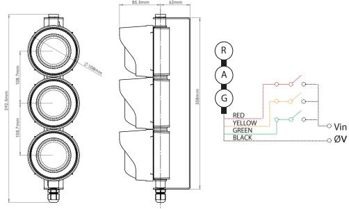
NOTE: For 48v DC Voltage Supply and above, reverse the polarity of "0v and +" for the PCB connections to allow for use on Direct Current supply.
