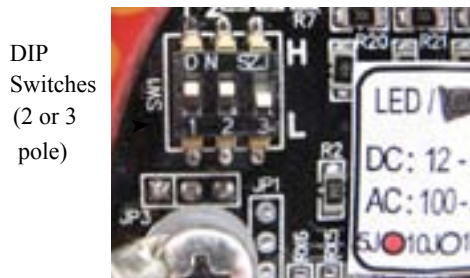
Picture 2 - TYPICAL COVER PCB
