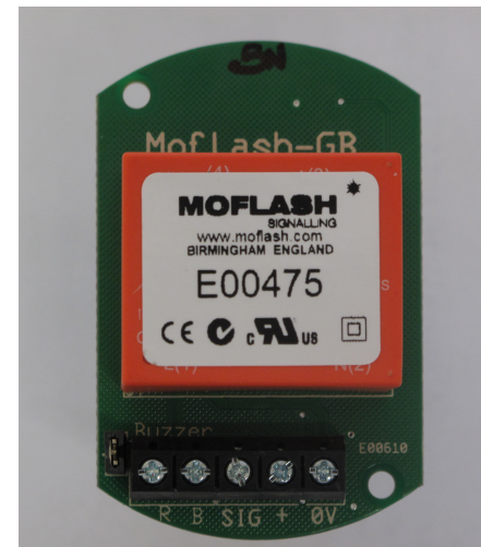
The above image shows the 115/230vAC PCB and is for illustration purposes only.
